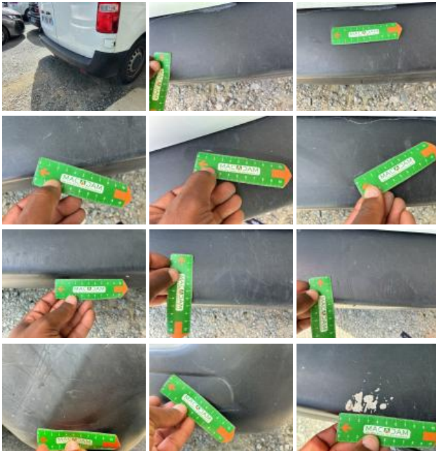
Boot door panel RL, Dent(s) and scratch(es), Repair and paint (complete)
