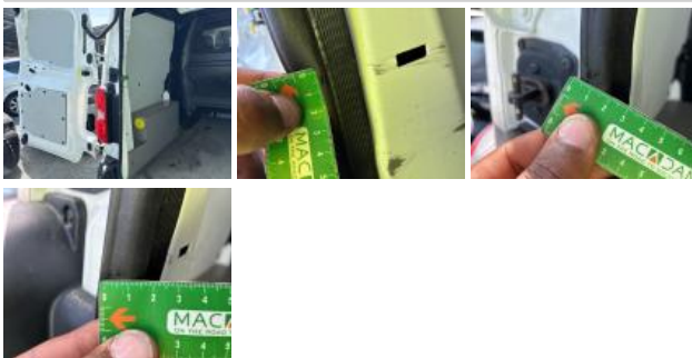
Rear light L, Scratch(es), Replace
