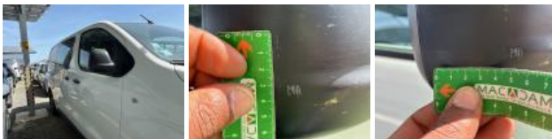
Outer sill R, Scratch(es), Acceptable
