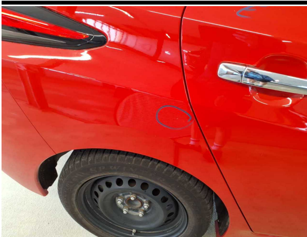
Damage #9: Side panel - rear right side: Side panel - Dent / paintcoat damage - Repair and paint
