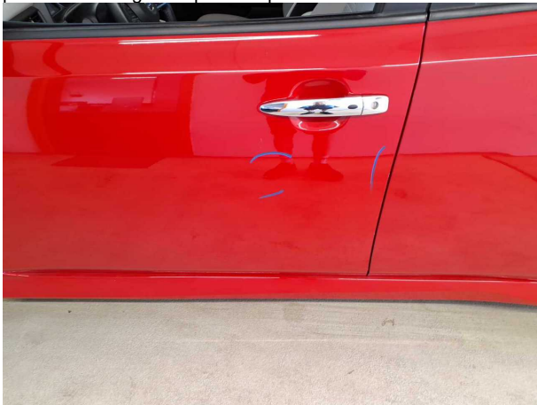
Damage #10: Door - front left side: Door - Scratched - Repair and paint
