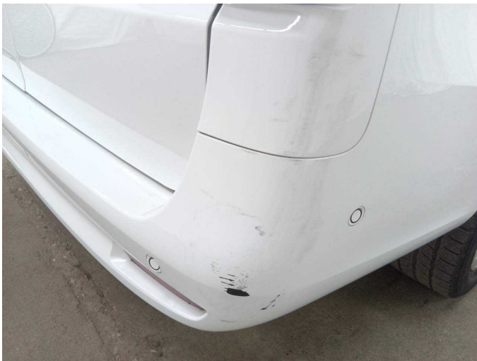
Damage 5: Rear bumper: Rear bumper - Scratch(es) - Paint
