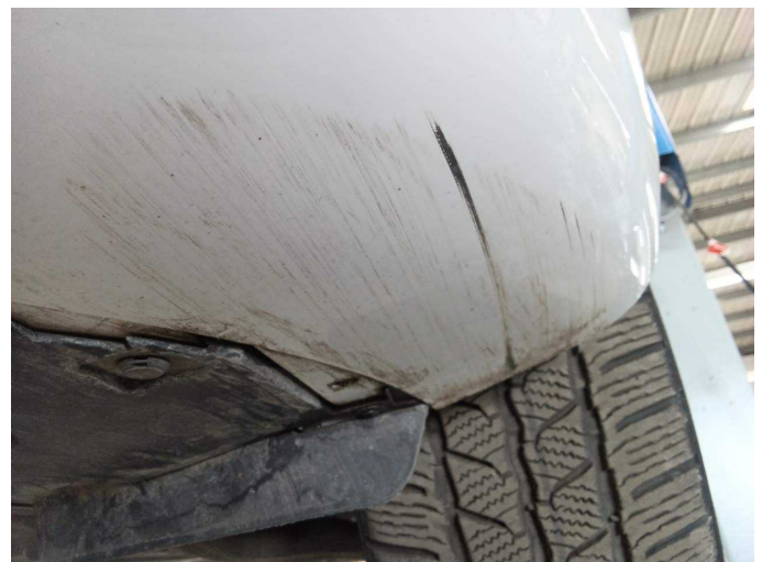
Damage 6: Front bumper: Front bumper - Scratch(es) - Paint
