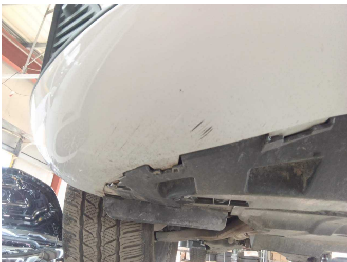
Damage 6: Front bumper: Front bumper - Scratch(es) - Paint
