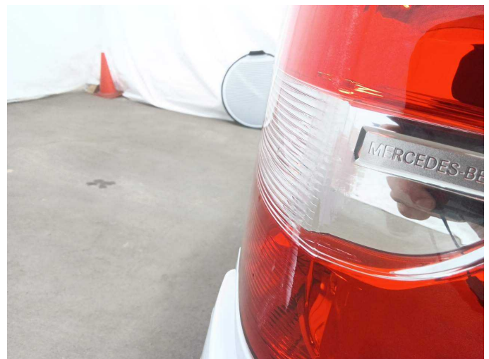
Damage 4: Tail light: Tail lamp - right side - Scratch(es) - Replace
