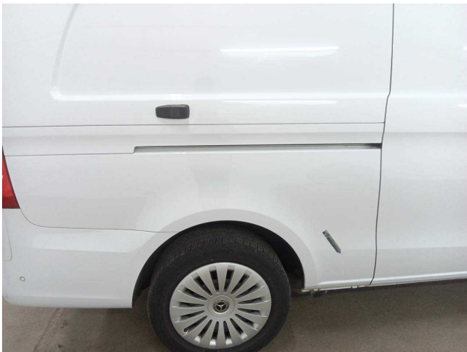
Damage 8: Side panel - rear right side: Side panel - Scratch(es) - Paint
