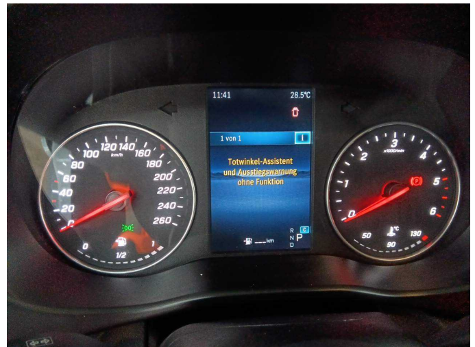
Damage 3: Instrument panel: Indicator light (Totwinkelassistent + Ausstiegswarnung) - on - Perform diagnosis
