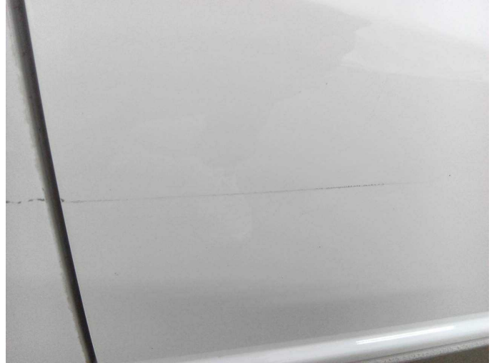
Damage 7: Sliding door, right: Sliding door - Scratch(es) - Paint
