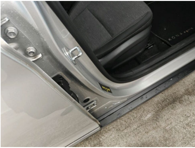
Door frame FR Dent(s) and scratch(es) Repair and paint (complete) Right
