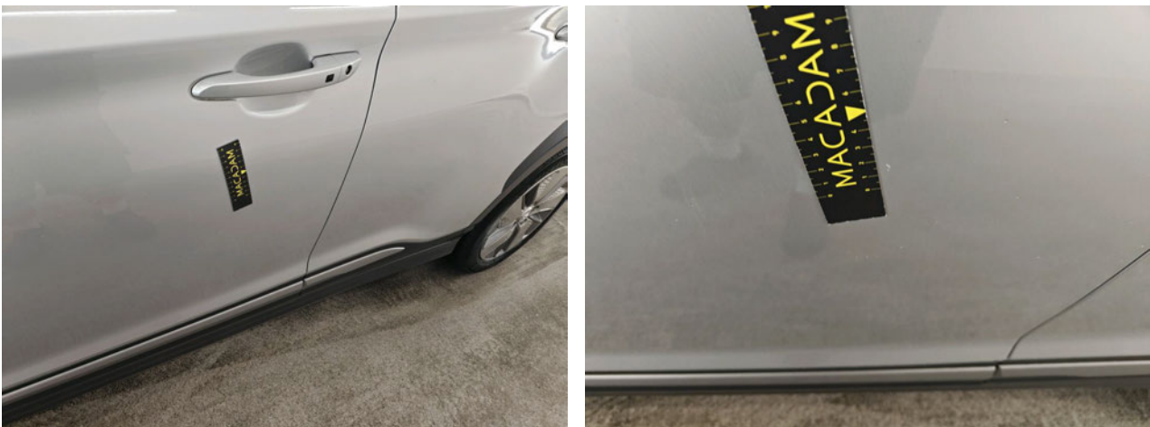
Door FL Scratch(es) Repair and paint (complete) Left
