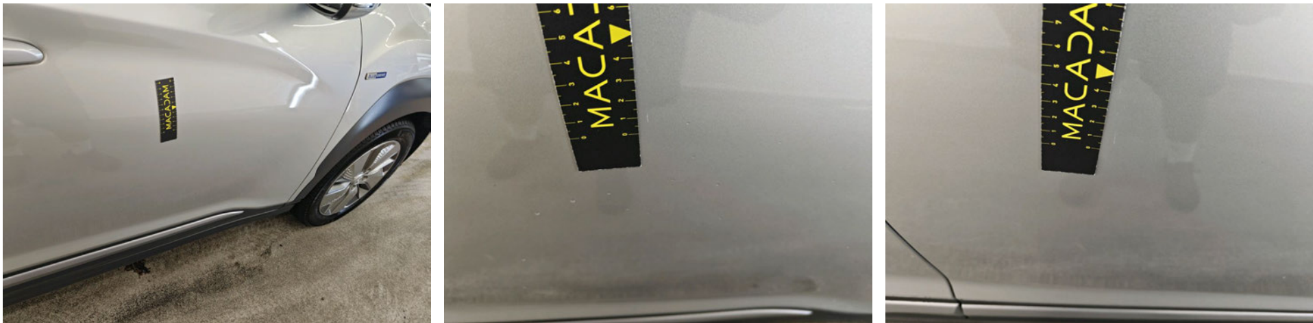
Door FR Scratch(es) Repair and paint (complete) Right
