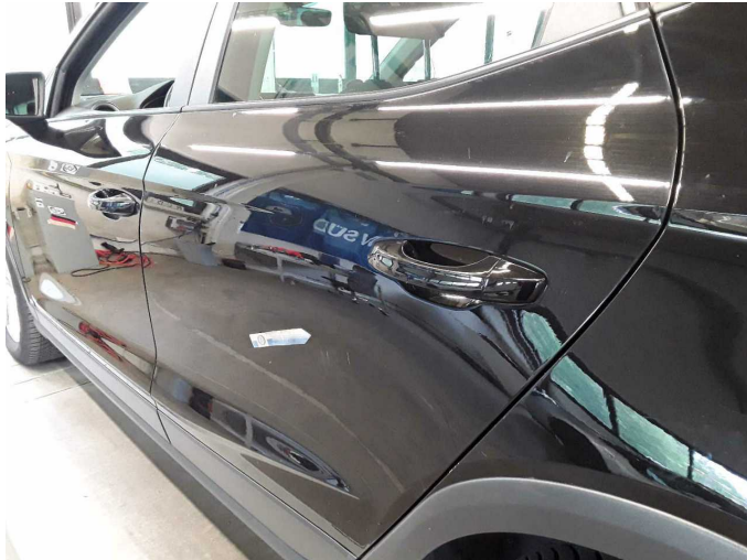
Damage 10: Door - rear left side: Door - Scratched - Paint
