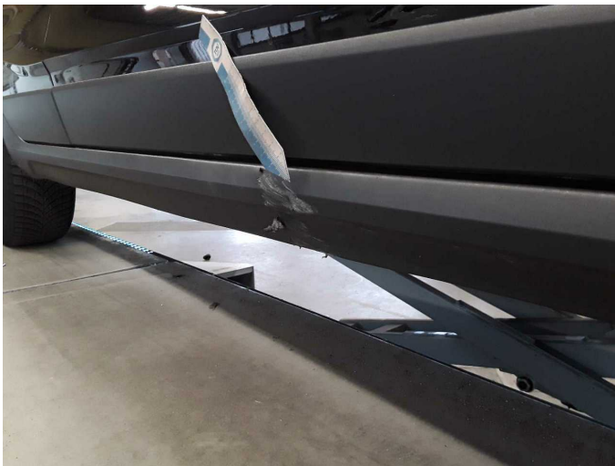
Damage 2: Sill - right side: Trim - Scratched - Replace
