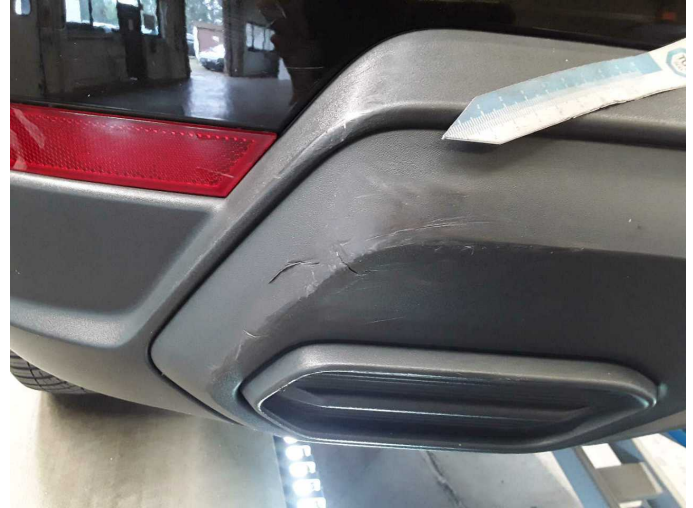
Damage 7: Rear bumper: Spoiler - Scratch(es) - Replace
