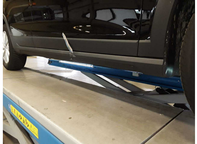
Damage 2: Sill - right side: Trim - Scratched - Replace
