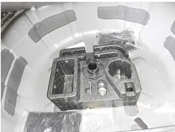
Missing part 1: Equipment: Tirefit compressor - Missing - Replace
