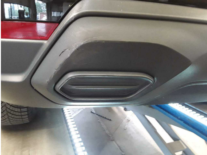
Damage 7: Rear bumper: Spoiler - Scratch(es) - Replace
