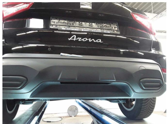
Damage 7: Rear bumper: Spoiler - Scratch(es) - Replace
