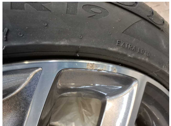
Damage 8: 2nd wheel set: 2 alloy rims (Materialabtrag) - Scratched - Replace
