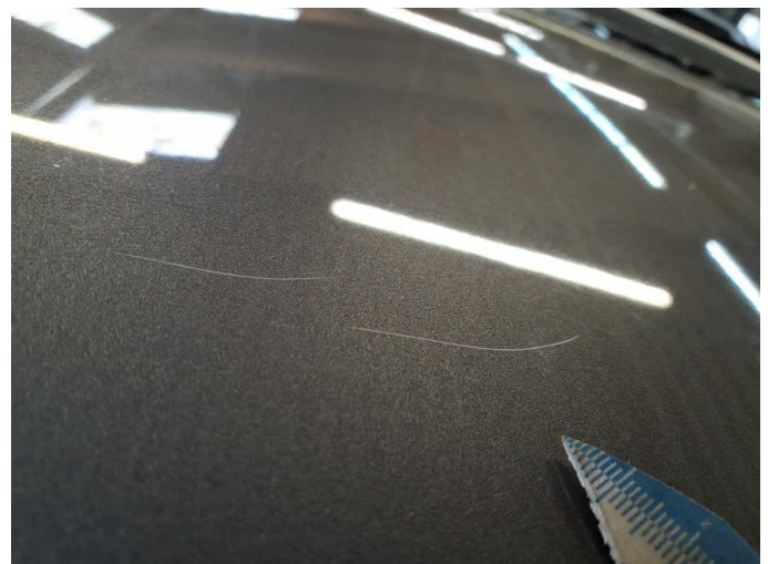
Damage 11: Roof: Roof - Scratch(es) - Paint
