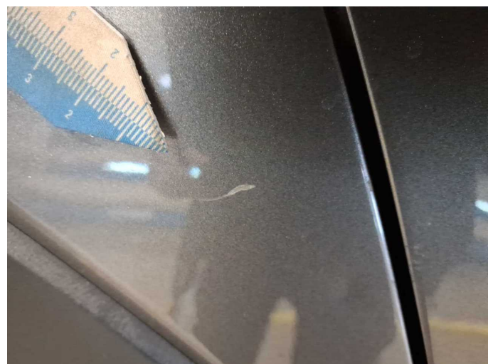
Damage 4: Side panel - rear right side: Side panel - Dent / paintcoat damage - Smart repair
