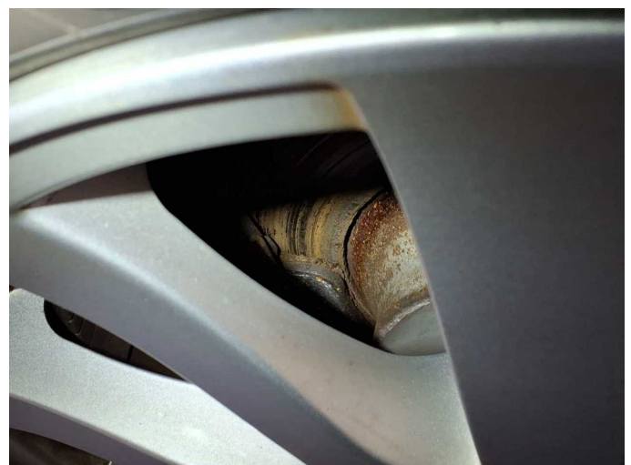
Damage 12: Braking system: Brake discs and brake pads - front (+ Hinten, schlechte Bremswirkung) - Corrosion - Replace
