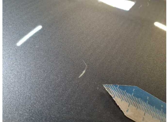
Damage 11: Roof: Roof - Scratch(es) - Paint
