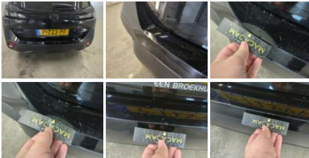
Bumper trim R, Dent(s) and scratch(es), Replace
