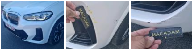
Bumper moulding F, Dent(s) and scratch(es), Replace
