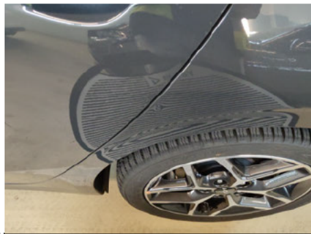
Kotflügel / Hinten Links / Delle
