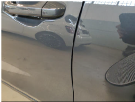
Tür / Vorne Links / Kratzer
