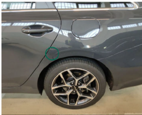
Kotflügel / Hinten Links / Delle
