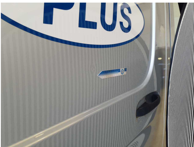
Damage 4: Sliding door, right: Sliding door - Dent / paintcoat damage - Repair and paint
