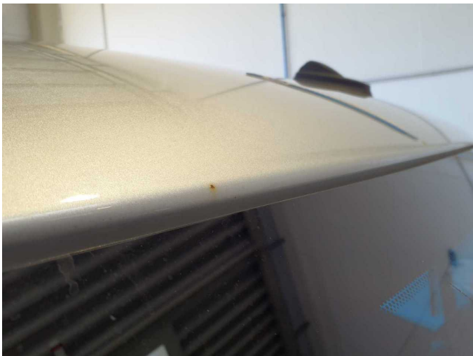
Damage 3: Roof: Roof - Corrosion - Repair and paint
