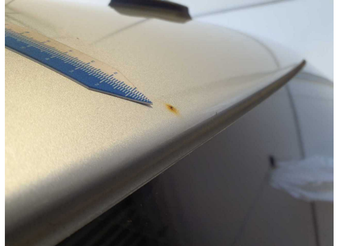
Damage 3: Roof: Roof - Corrosion - Repair and paint
