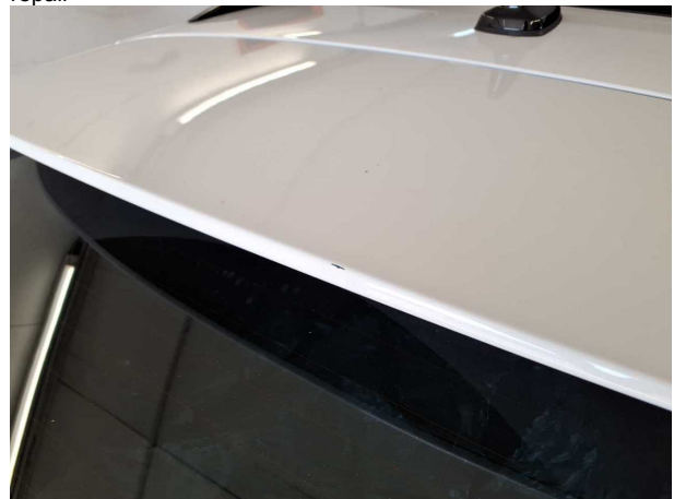
Damage #12: Boot lid / rear door: Rear spoiler - Scratched - Smart repair
