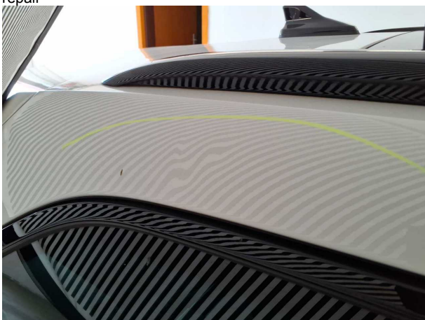
Damage #13: Roof: Roof rail - right side - dent(s) - Smooth repair work
