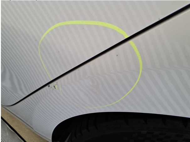
Damage #14: Side panel - rear left side: Side panel - dent(s) - Repair and paint
