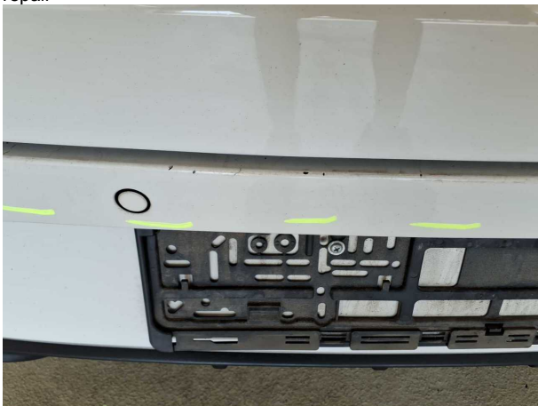
Damage #11: Rear bumper: Rear bumper - Scratched - Smart repair
