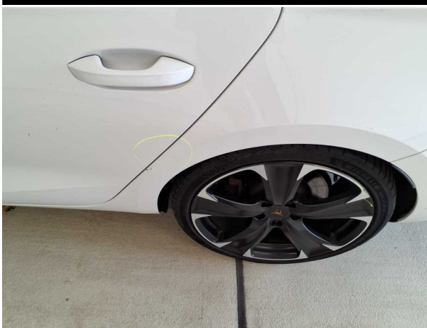
Damage #14: Side panel - rear left side: Side panel - dent(s) - Repair and paint
