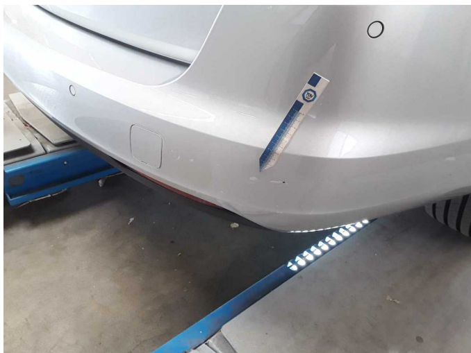
Damage 5: Rear bumper: Rear bumper - Scratched - Paint
