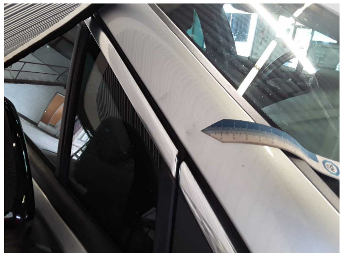
Damage 3: Body: A-pillar - right side - dent(s) - Smart repair
