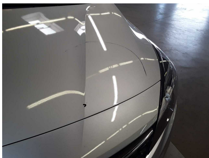
Damage 9: Bonnet: Bonnet - Stone chips - Paint
