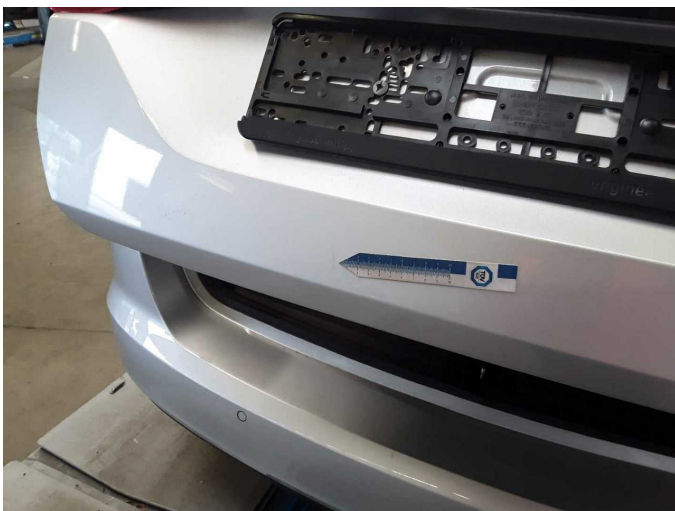
Damage 2: Boot lid / rear door: Boot lid - Scratch(es) - Smart repair
