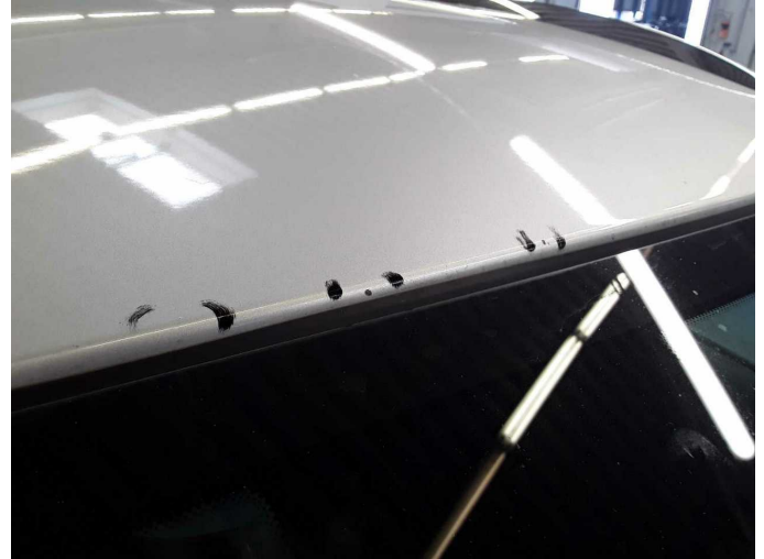
Damage 10: Roof: Roof - Stone chips - Paint
