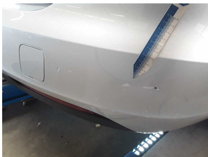
Damage 5: Rear bumper: Rear bumper - Scratched - Paint
