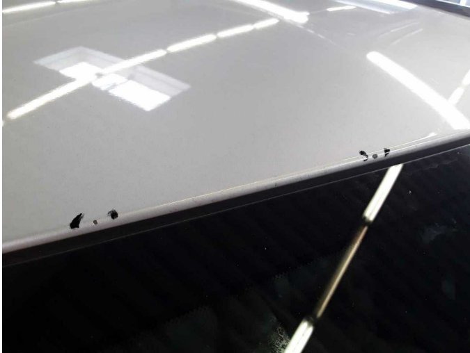
Damage 10: Roof: Roof - Stone chips - Paint
