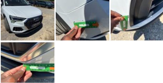
Bumper F, Scratch(es), Repair and paint (complete)
