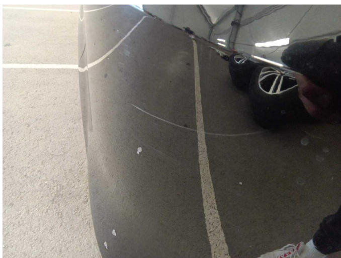
Damage 4: Rear bumper: Rear bumper - Scratch(es) - Paint
