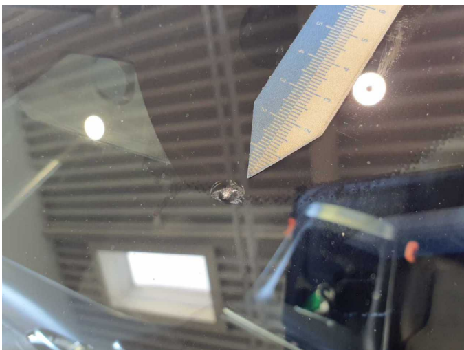
Damage 4: Vehicle glazing: Windscreen - Stone chips - Replace
