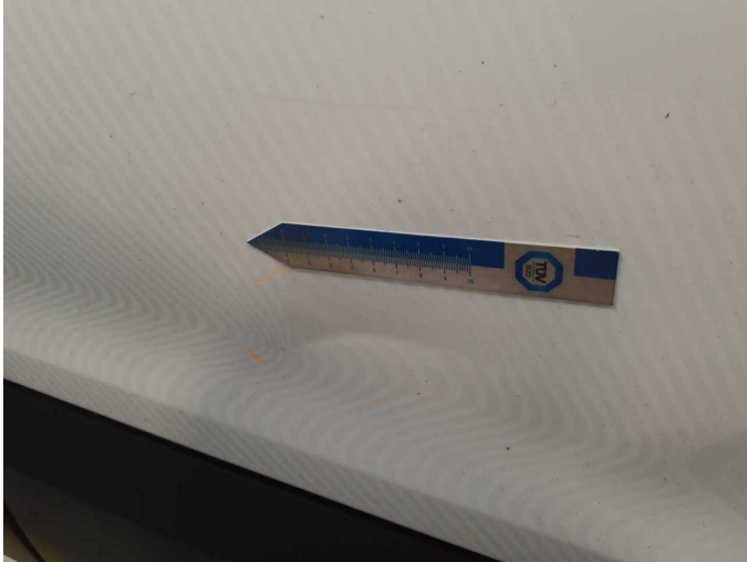
Damage 8: Door - front right side: Door (unterhalb) - Deformed - Repair and paint
