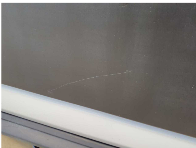
Wear and tear 4: Sliding door, right: Sliding door (Zierleiste) - Scratch(es) - No deduction
