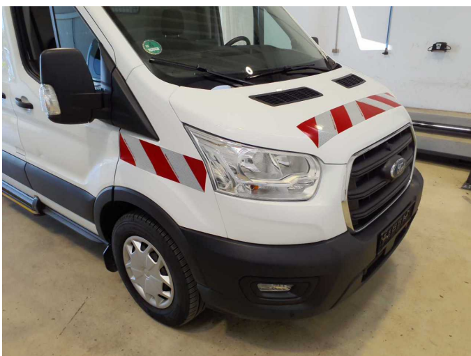
Damage 6: Body: Body - Glued / labelled - De-glug / neutralise
