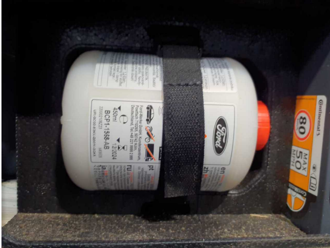
Damage 1: Equipment: Tirefit filler - Expired - Replace
