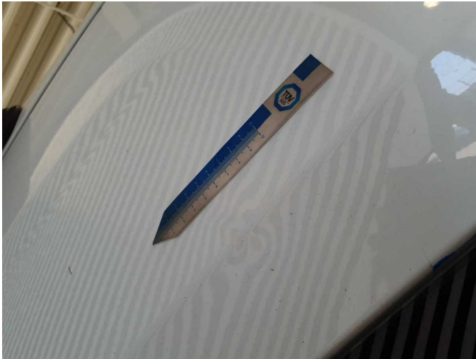
Damage 3: Boot lid / rear door: Rear door - right side - dent(s) - Smart repair
