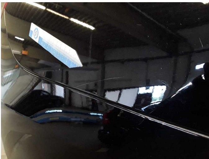
Damage 5: Side panel - rear right side: Side panel - Dent / paintcoat damage - Repair and paint
