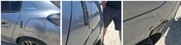
Door RL, Dent(s), Repair and paint (complete)
