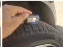
Tyre RR, Out of tolerance, Replace
