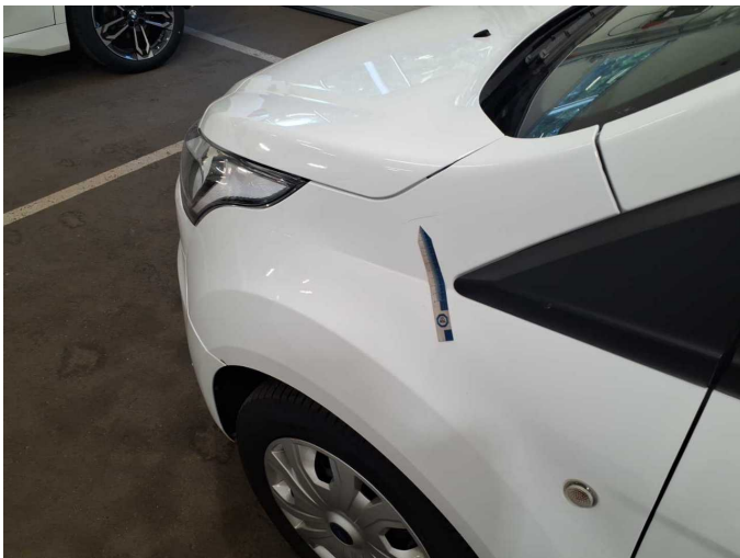
Damage 4: Mudguard - left side: Mudguard - left side - Scratch(es) - Paint
