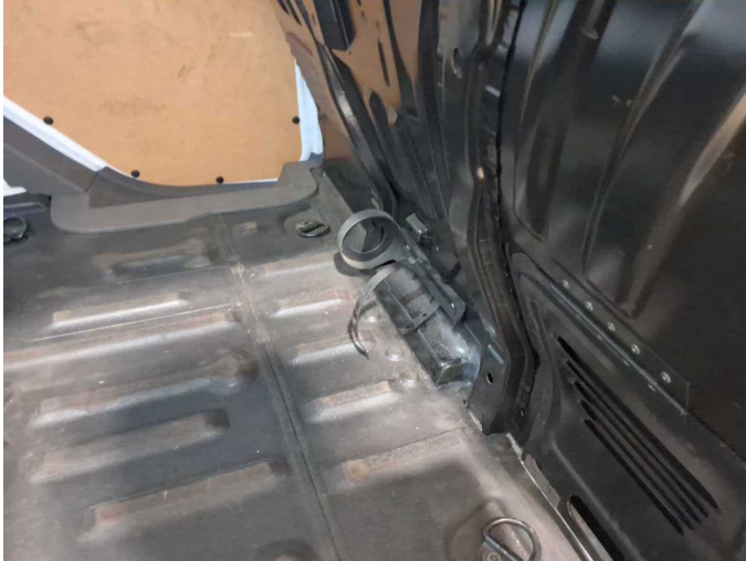
Missing part 1: Equipment: Fire extinguisher - Missing - Replace
