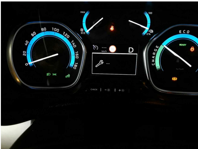
Damage 7: Misc.: Inspection / maintenance - Due - Perform
