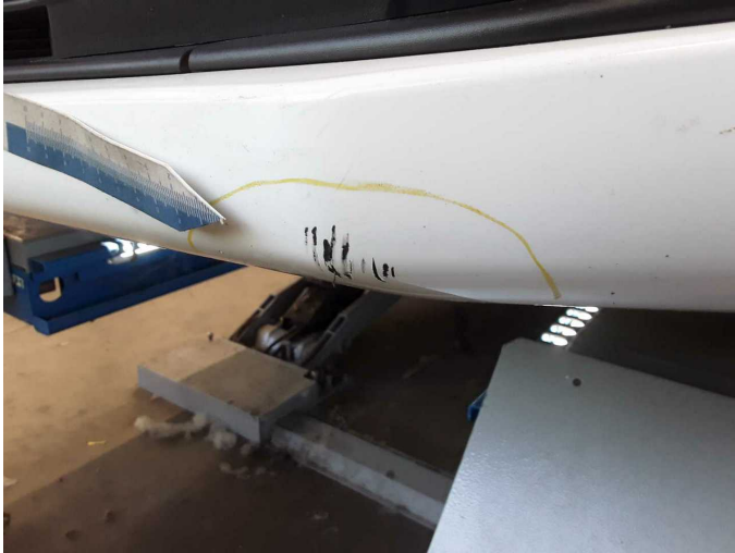
Damage 9: Front bumper: Front bumper - Scratch(es) - Paint
