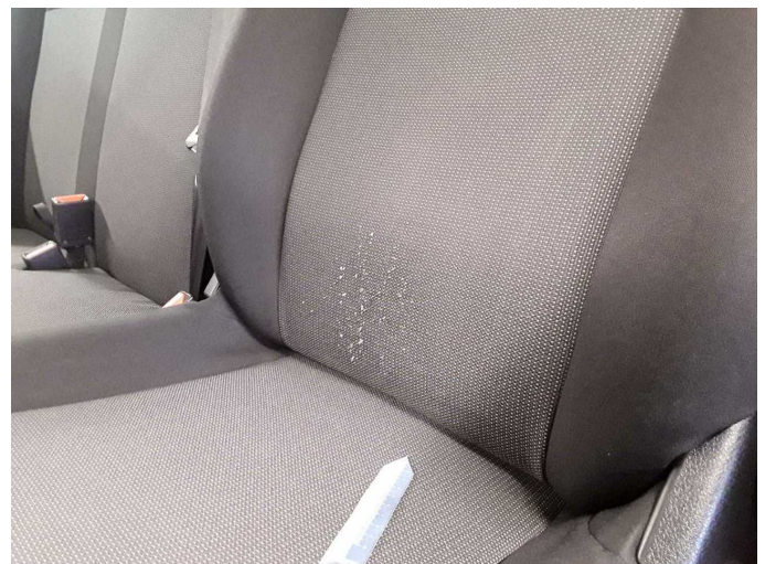
Damage 5: Seat - front: Backrest cover - left side - Worn - Smart repair
