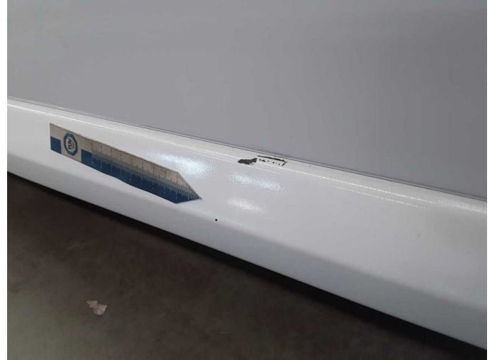
Damage 3: Door - front right side: Brightware - lower - Scratch(es) - Smart repair
