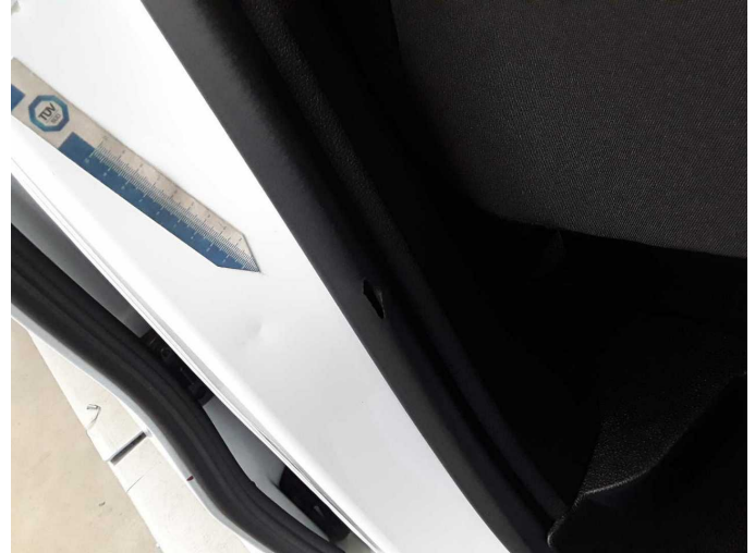
Damage 6: Cab: Door rubber seal - right side - Damaged - Replace
