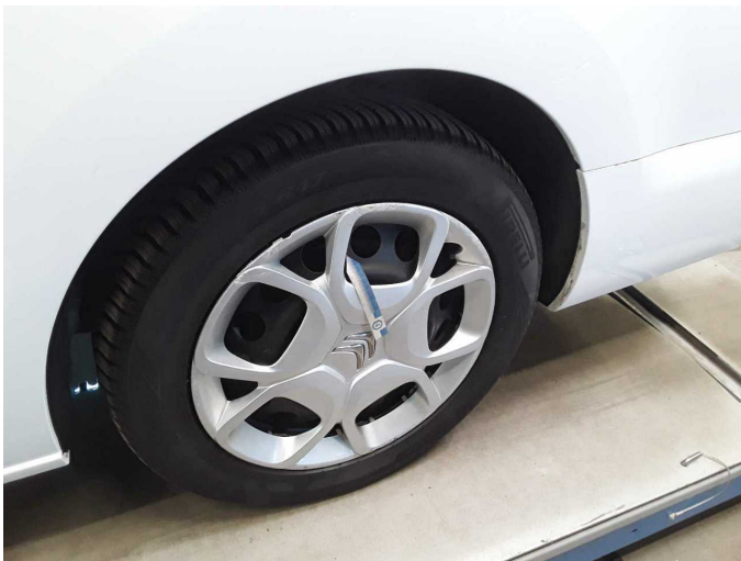
Damage 1: Wheel / tyres: Wheel cover - rear left side - Damaged - Replace
