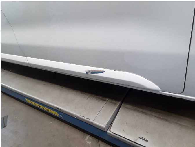
Damage 4: Door - rear left side: Brightware - lower - Scratched - Smart repair
