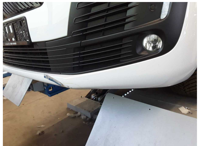
Damage 9: Front bumper: Front bumper - Scratch(es) - Paint
