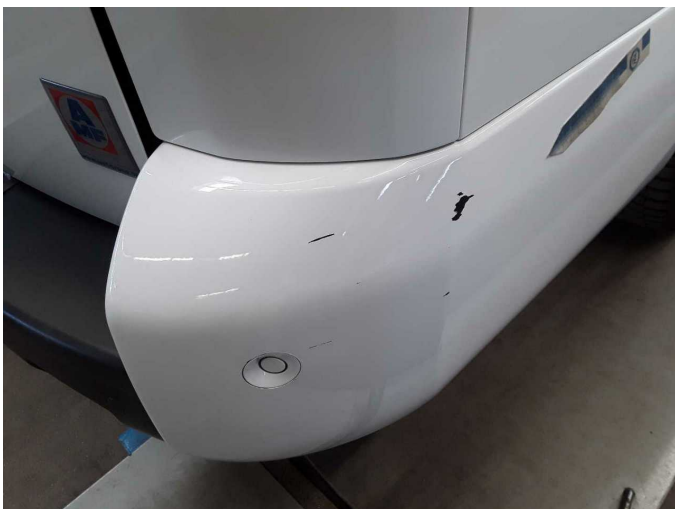
Damage 8: Rear bumper: Rear bumper - Scratch(es) - Paint
