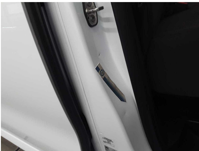
Damage 2: Sill - right side: Sill - Dent / paintcoat damage - Smart repair
