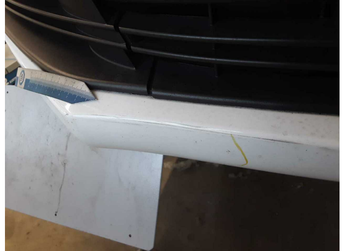
Damage 9: Front bumper: Front bumper - Scratch(es) - Paint
