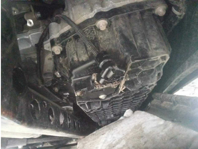
Damage 8: Engine: Engine oil sump (Ölstandsensord/Ölqualitätsensord) - Broken / torn - Replace
