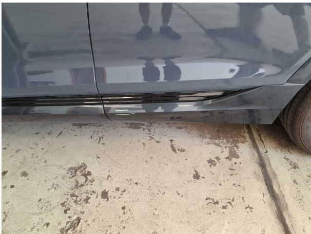
Damage #4: Door - rear left side: Brightware - lower - Abrasion - Cover / polish
