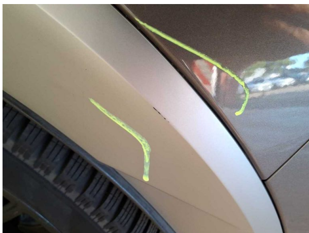
Damage #6: Side panel - rear left side: Wheel well extension - Scratched - Loss in value
