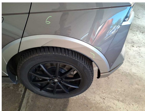
Damage #6: Side panel - rear left side: Wheel well extension - Scratched - Loss in value
