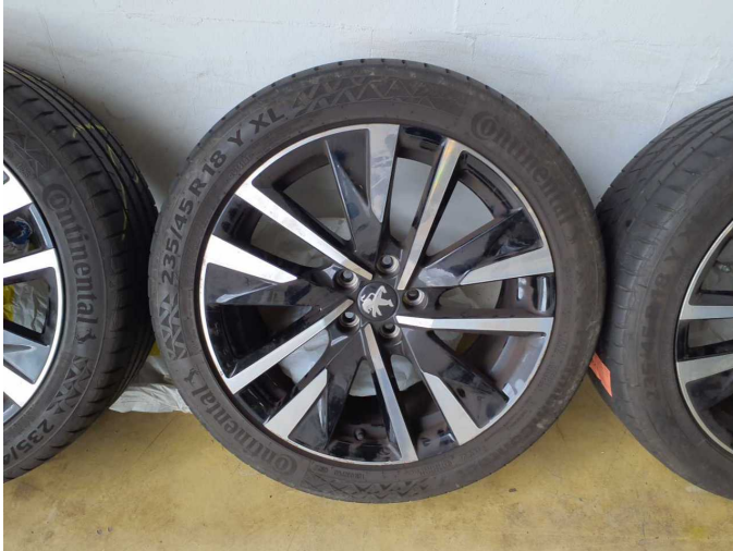
Damage 7: 2nd wheel set: 1 tyre - Porous / cracked - Replace
