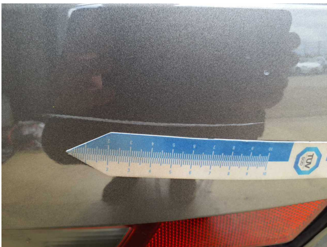
Damage 13: Rear bumper: Rear bumper - Scratch(es) - Paint
