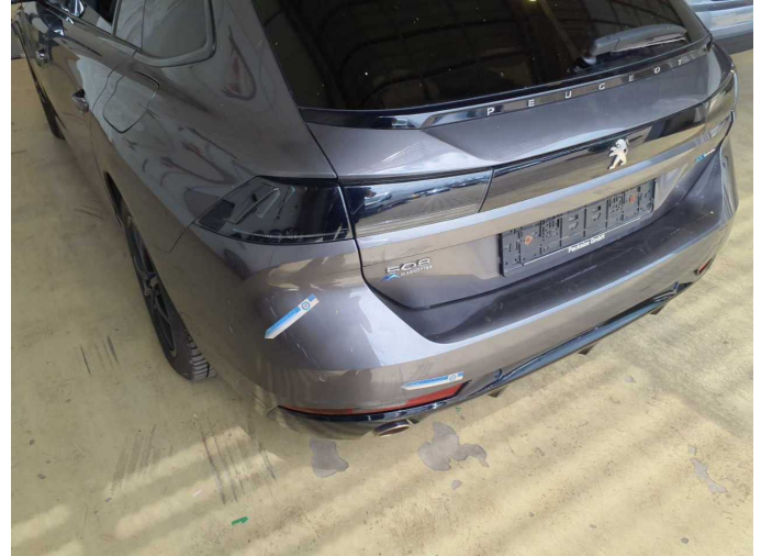
Damage 13: Rear bumper: Rear bumper - Scratch(es) - Paint
