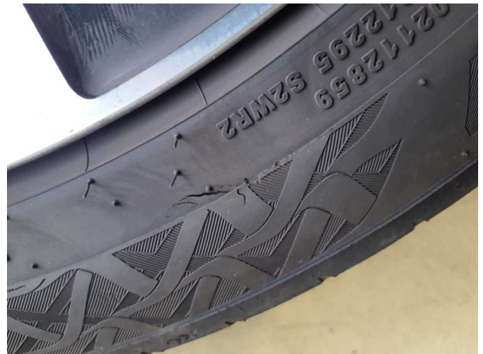
Damage 8: 2nd wheel set: 1 tyre - Porous / cracked - Replace
