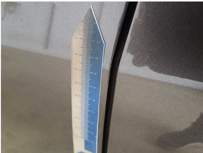
Damage 5: Door - front left side: Door edge - Scratch(es) - Smart repair
