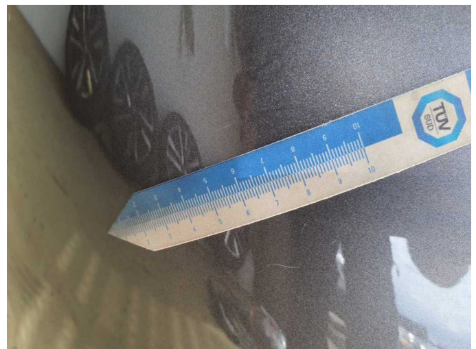
Damage 13: Rear bumper: Rear bumper - Scratch(es) - Paint
