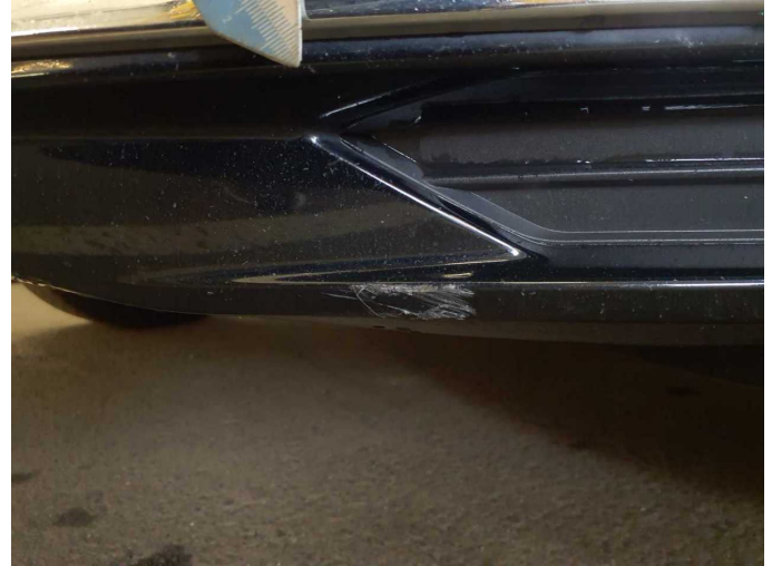
Damage 4: Front bumper: Front bumper - Scratch(es) - Paint
