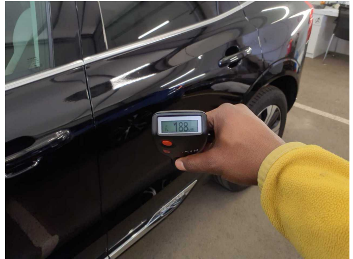
Repainting 1: Door - rear left side
