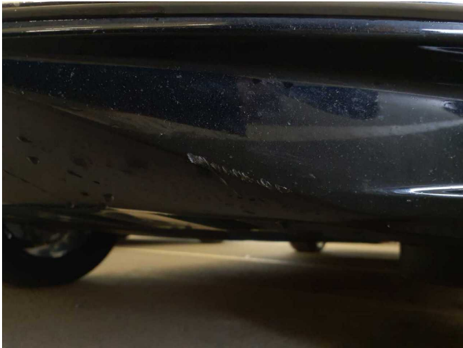
Damage 4: Front bumper: Front bumper - Scratch(es) - Paint
