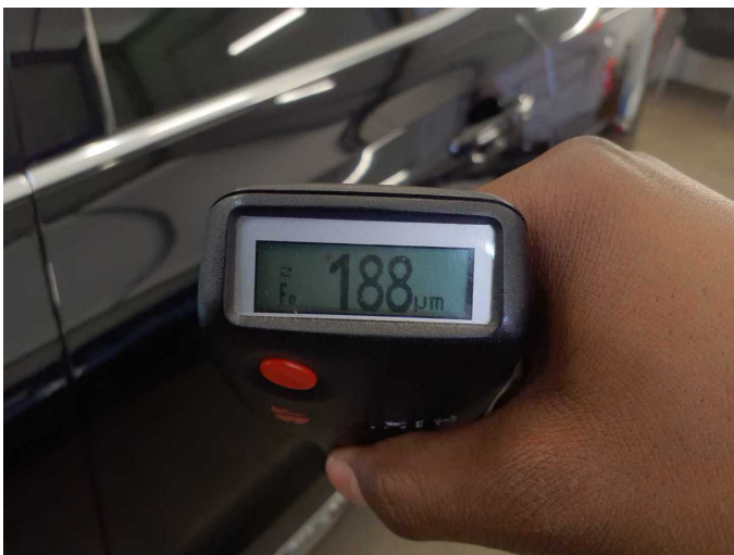
Repainting 1: Door - rear left side
