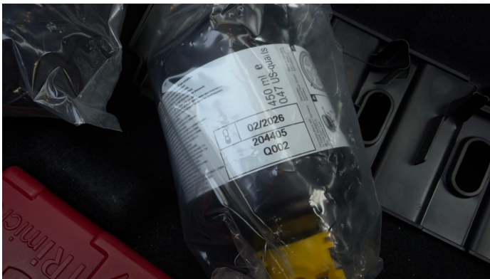
Damage 1: Equipment: Tirefit filler - Expired - Replace
