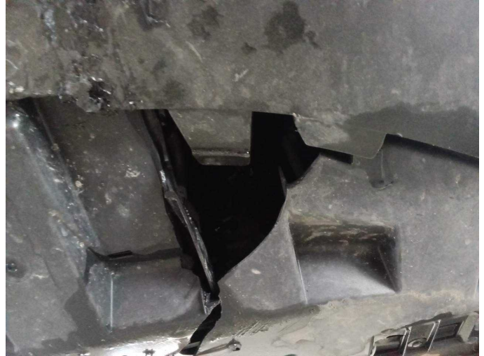
Damage 2: Body: Underbody panelling - Broken / torn - Replace
