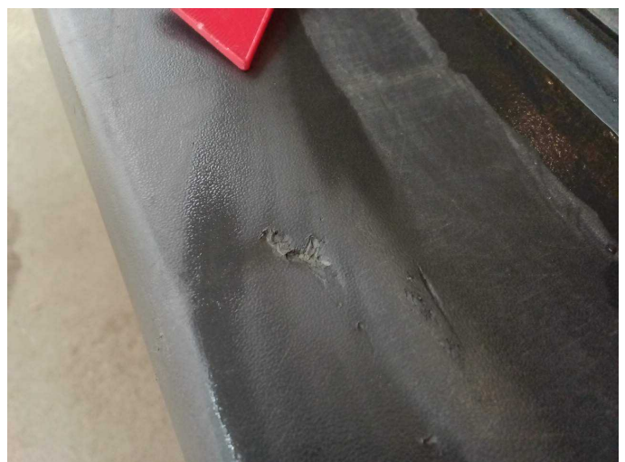
Damage 6: Rear bumper: Rear bumper - Scratched - Replace
