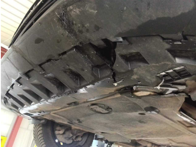
Damage 2: Body: Underbody panelling - Broken / torn - Replace
