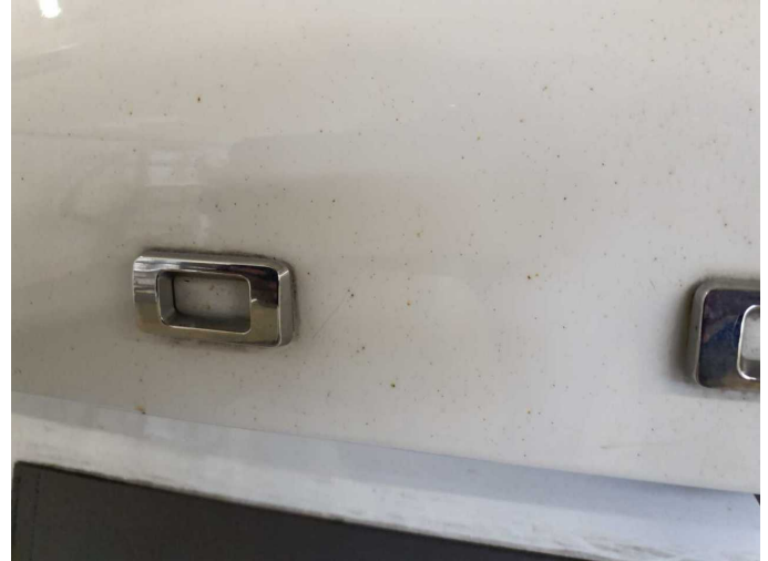
Damage 3: Body: Body (Flugrost) - Soiled - Clean
