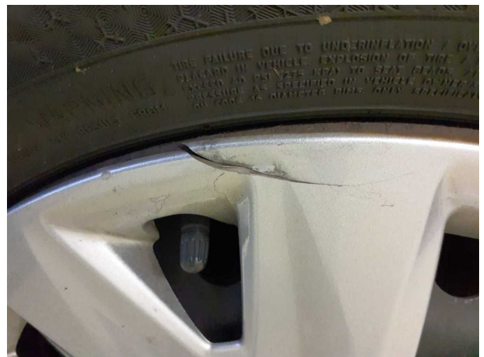
Damage 1: Wheel / tyres: Wheel cover - front left side - Broken / torn - Replace
