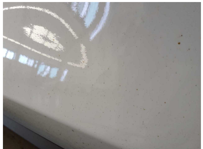
Damage 3: Body: Body (Flugrost) - Soiled - Clean
