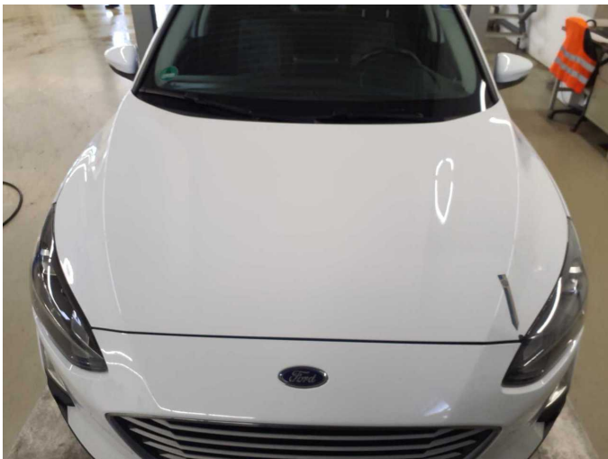
Damage 4: Bonnet: Bonnet (+ Korrosion) - Paint defect - Repair and paint
