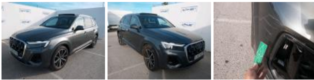
Bumper F, Scratch(es), Repair and paint (complete)
