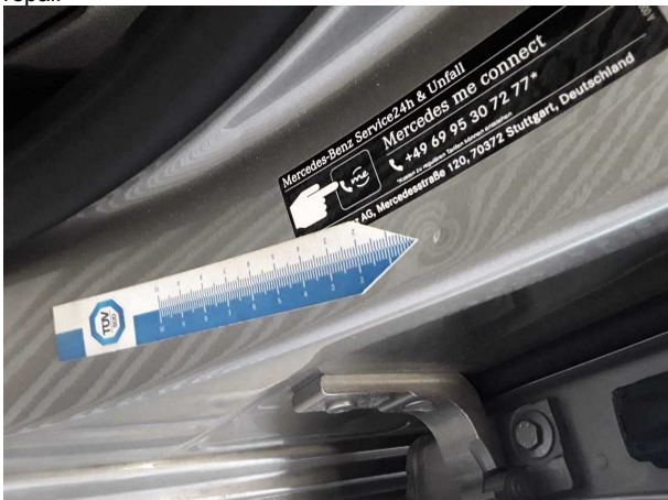
Damage #1: Sill - left side: Sill - Dent / paintcoat damage - Smart repair
