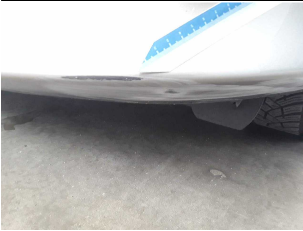
Damage #5: Front bumper: Front bumper - Scratched - Repair and paint
