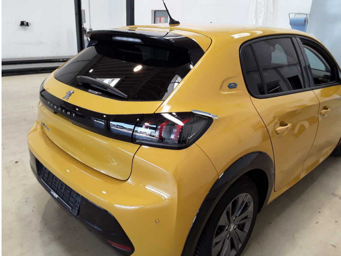
Damage 1: Tail light: Tail lamp - right side (Randbereich) - Scratched - Replace
