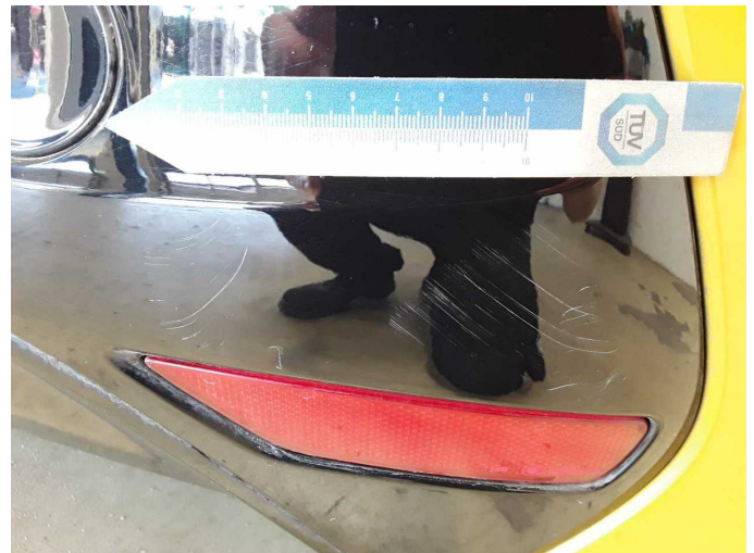
Damage 2: Rear bumper: Spoiler - Scratch(es) - Paint
