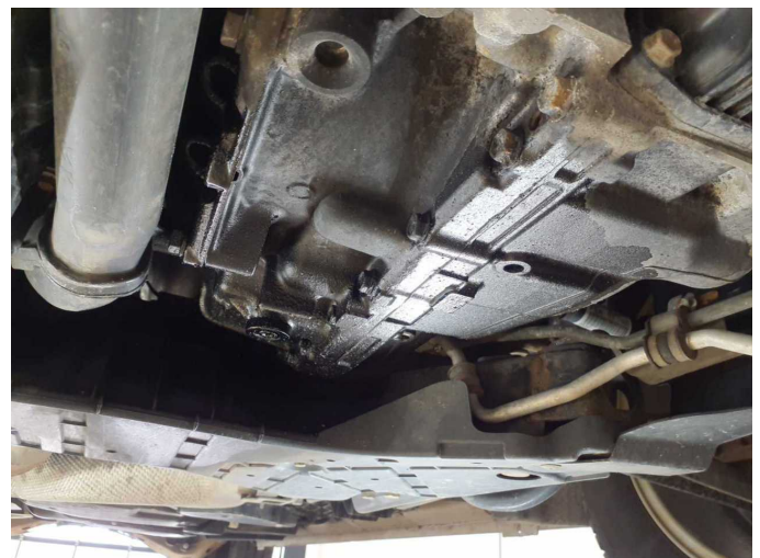
Damage 3: Gearbox: Gearbox - Leaking - Perform diagnosis
