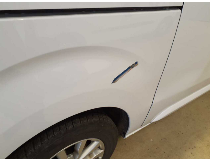
Damage 6: Side panel - rear right side: Side panel - dent(s) - Smooth repair work
