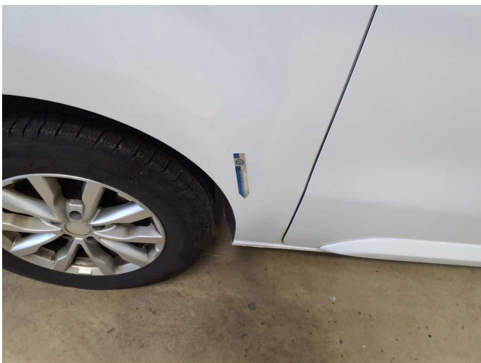
Damage 9: Side panel - rear right side: Side panel - Scratch(es) - Smart repair
