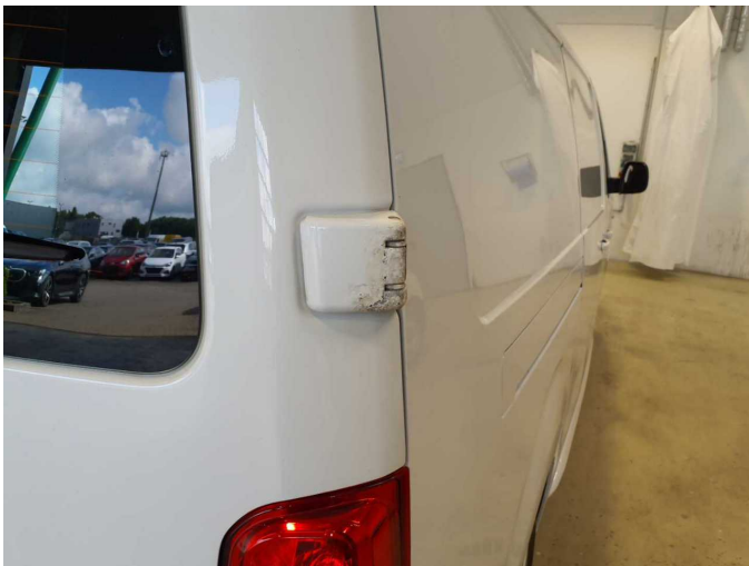
Damage 11: Boot lid / rear door: Hinge (Lack löst sich) - Paint defect - Smart repair
