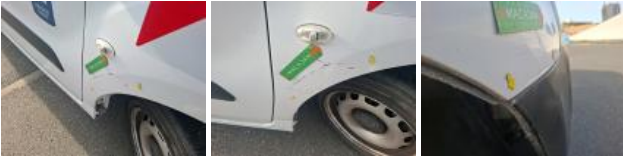
Wing FR, Dent(s) and scratch(es), Repair and paint (complete)
