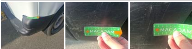
Bumper corner RR, Scratch(es), Repair and paint (complete)
