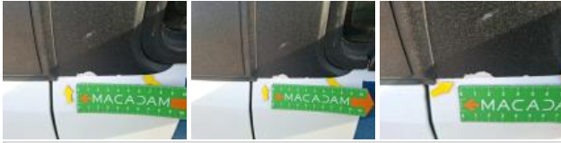
Outer sill L, Dent(s) and scratch(es), Repair and paint (complete)
