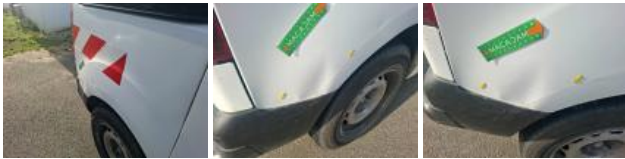
Sliding door R, Dent(s) and scratch(es), Repair and paint (complete)
