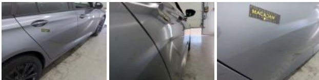
Wing RR, Dent(s), Repair and paint (complete)
