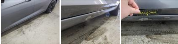
Door FL, Scratch(es), Repair and paint (complete)
