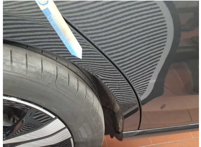
Damage 1: Side panel - rear right side: Elbow - dent(s) - Smooth repair work
