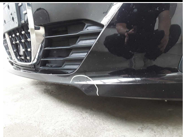
Damage #4: Front bumper: Spoiler - Scratched - Smart repair
