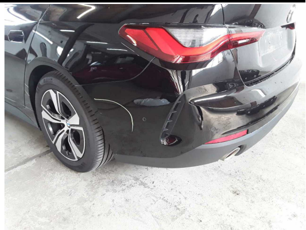
Damage #6: Rear bumper: Rear bumper - Scratched - Paint
