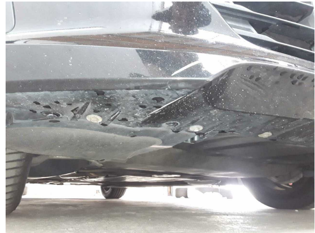
Damage #4: Front bumper: Spoiler - Scratched - Smart repair
