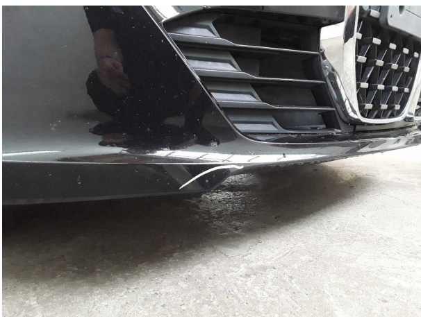
Damage #4: Front bumper: Spoiler - Scratched - Smart repair
