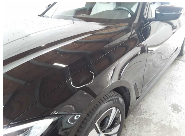
Damage #5: Mudguard - left side: Mudguard - left side - Scratch(es) - Paint
