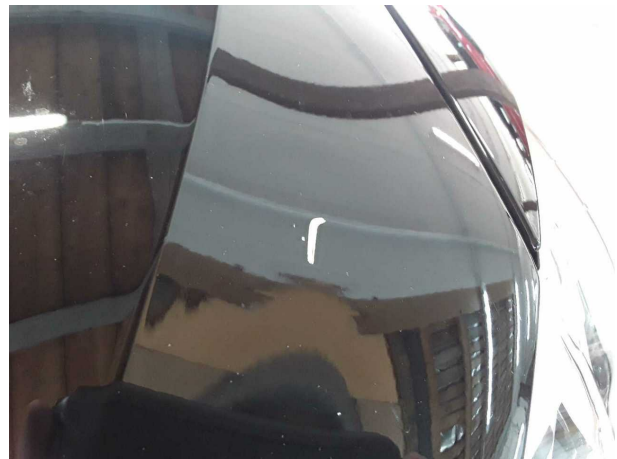
Damage #1: Bonnet: Bonnet - Stone chips - Cover / polish
