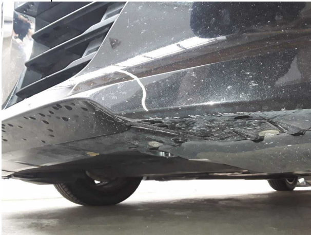
Damage #4: Front bumper: Spoiler - Scratched - Smart repair
