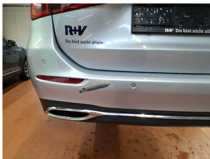
Wear and tear 4: Rear bumper: Rear bumper (Verladebereich) - Scratch(es) - No deduction
