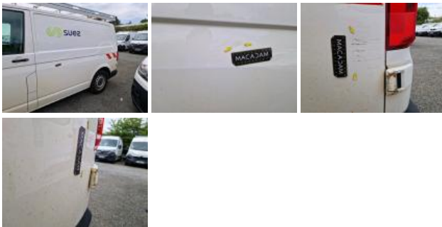
Brand badge F, Missing, Replace
