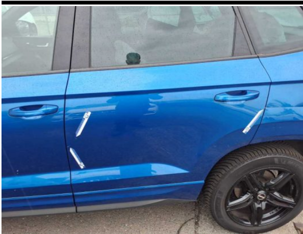
Damage #6: Door - rear left side: Door - Scratched - Repair and paint
