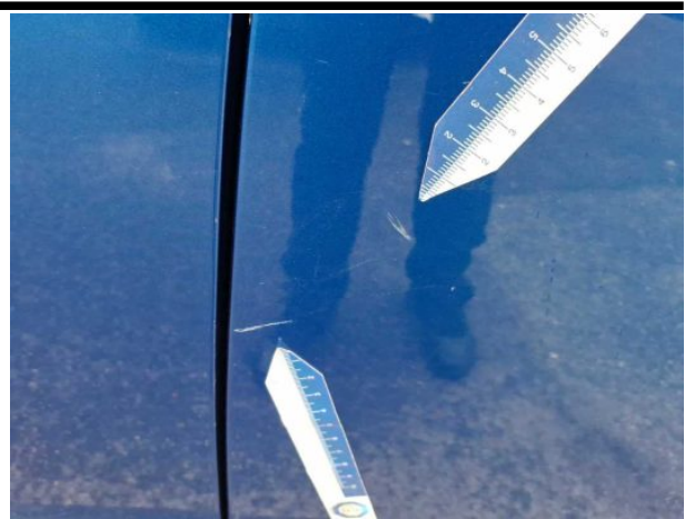
Damage #6: Door - rear left side: Door - Scratched - Repair and paint
