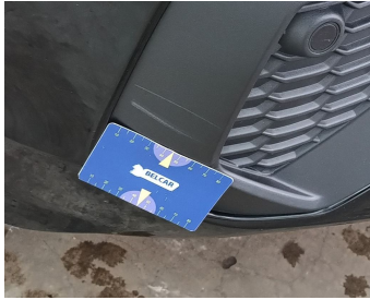
Bumper Front / Grid Right / Replace-scratch
