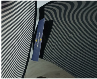
Wing Front right // Smart Repair Small-dent
