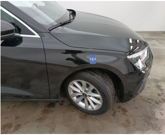
Wing Front right // Smart Repair Small-dent
