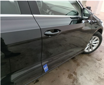
Door Front Right // Painting-scratch
