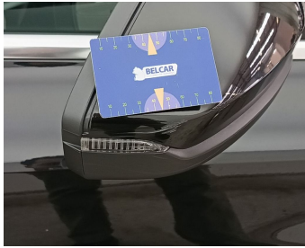
Side View Mirror Right // Painting-scratch
