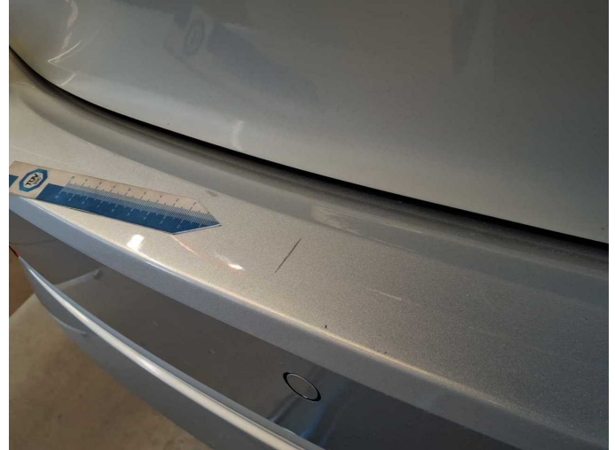
Damage 6: Rear bumper: Rear bumper - Scratch(es) - Paint
