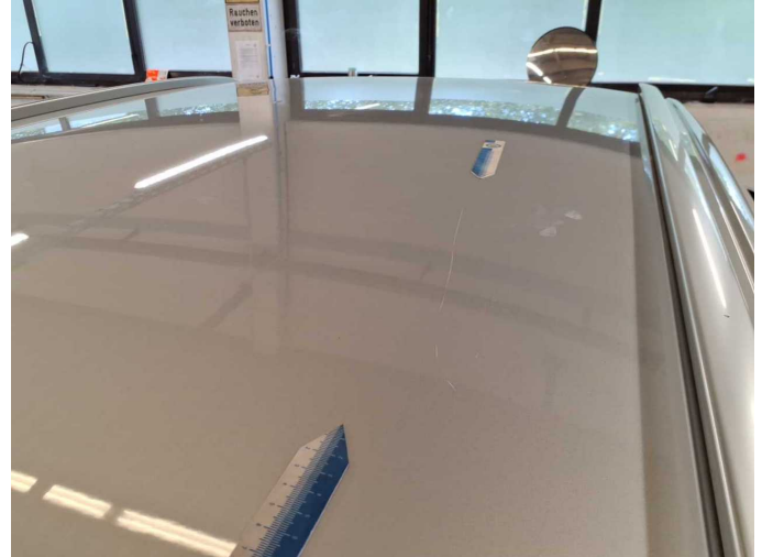
Damage 10: Roof: Roof - Scratch(es) - Paint
