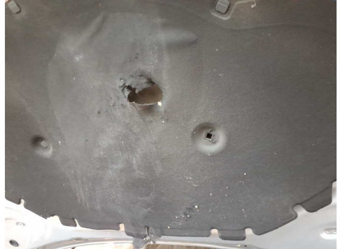
Damage 1: Bonnet: Insulation lining - Damaged - Replace
