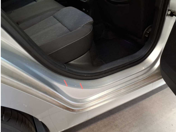
Wear and tear 4: Side panel - rear right side: Sill - Scratch(es) - Smart repair
