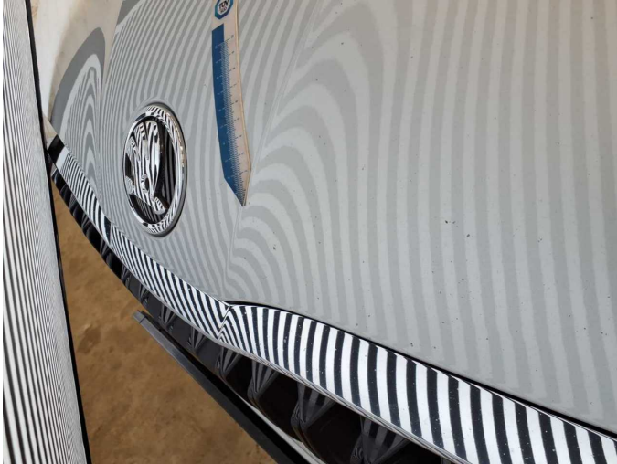
Damage 8: Bonnet: Bonnet - Dent / paintcoat damage - Paint
