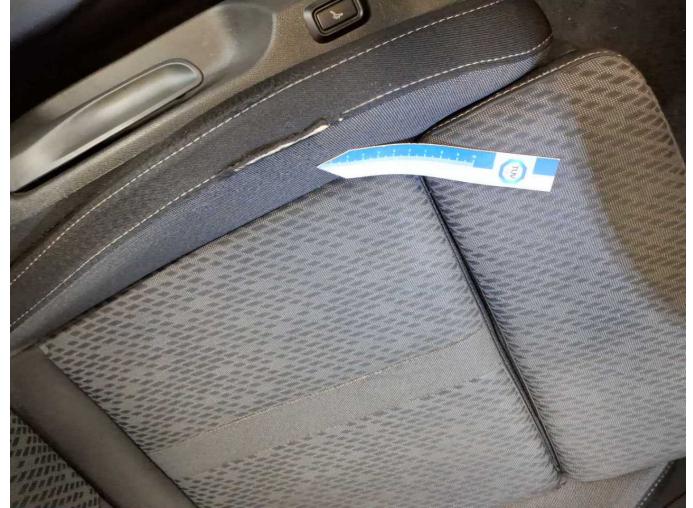
Damage 4: Seat - front: Seat cover - left side - Broken / torn - Smart repair
