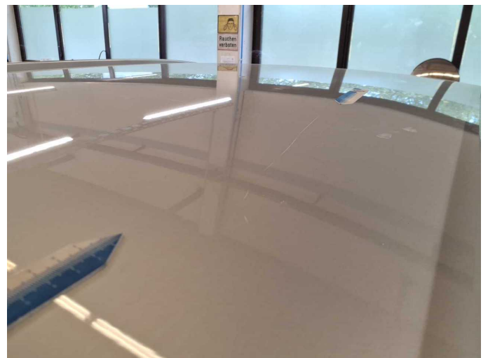
Damage 10: Roof: Roof - Scratch(es) - Paint
