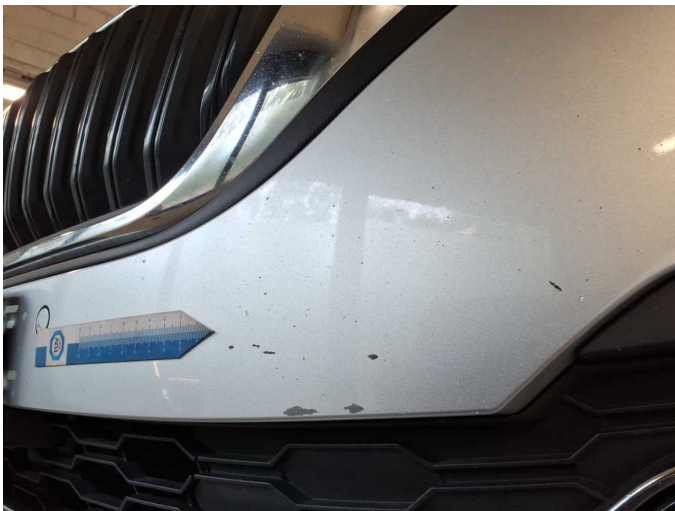
Damage 9: Front bumper: Front bumper - Scratch(es) - Paint
