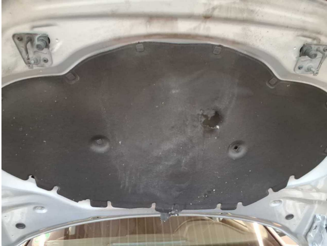
Damage 1: Bonnet: Insulation lining - Damaged - Replace
