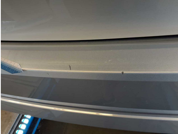
Damage 6: Rear bumper: Rear bumper - Scratch(es) - Paint
