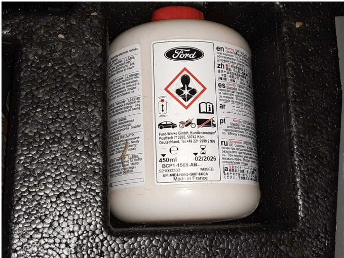
Damage 1: Equipment: Tirefit filler - Expired - Replace
