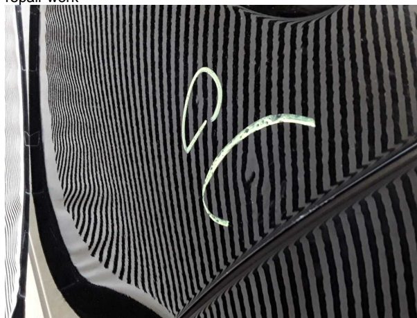
Damage #7: Door - front left side: Door - dent(s) - Smooth repair work
