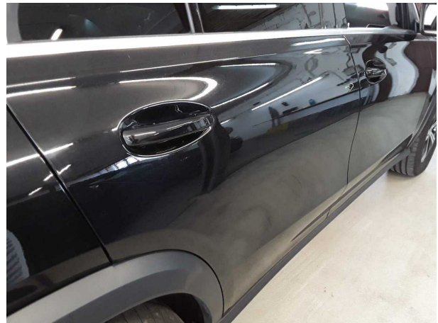
Damage #4: Door - rear right side: Door - Scratch(es) - Cover / polish
