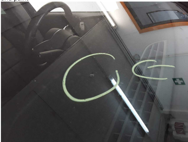
Damage #9: Vehicle glazing: Windscreen (Rissbildung) - Stone chips - Replace
