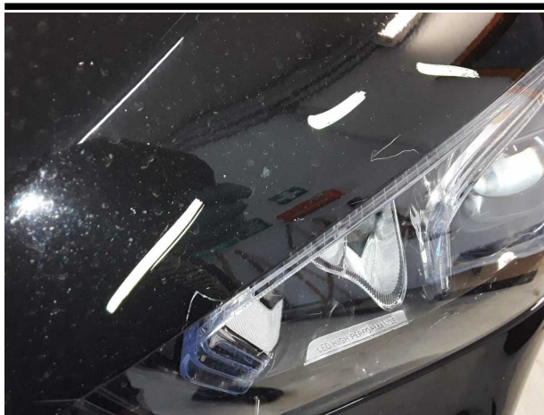
Damage #6: Bonnet: Bonnet - Scratched - Smart repair
