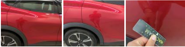
Wing RR, Dent(s), Repair and paint (complete)
