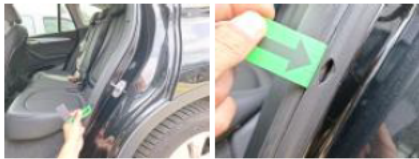
Wing trim RL, Scratch(es), Replace
