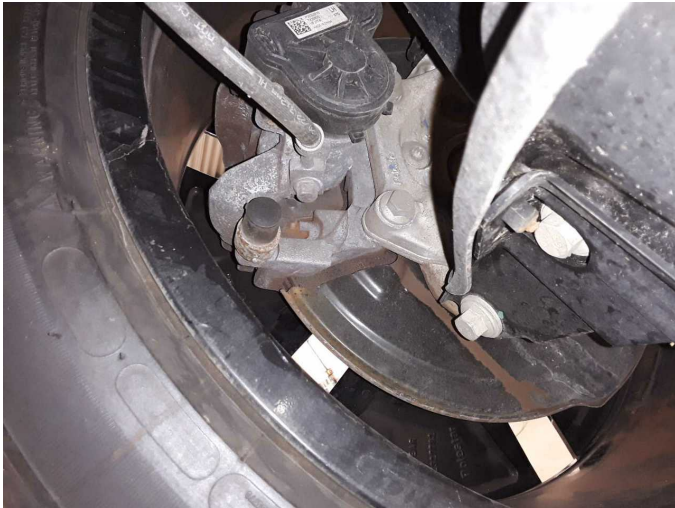
Damage 2: Braking system: Brake discs and pads - rear - Corrosion - Replace
