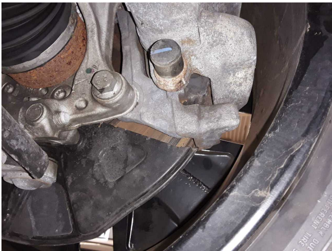
Damage 3: Braking system: Brake discs and brake pads - front - Corrosion - Replace
