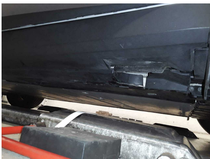
Damage 1: Body: Underbody panelling - Broken / torn - Replace
