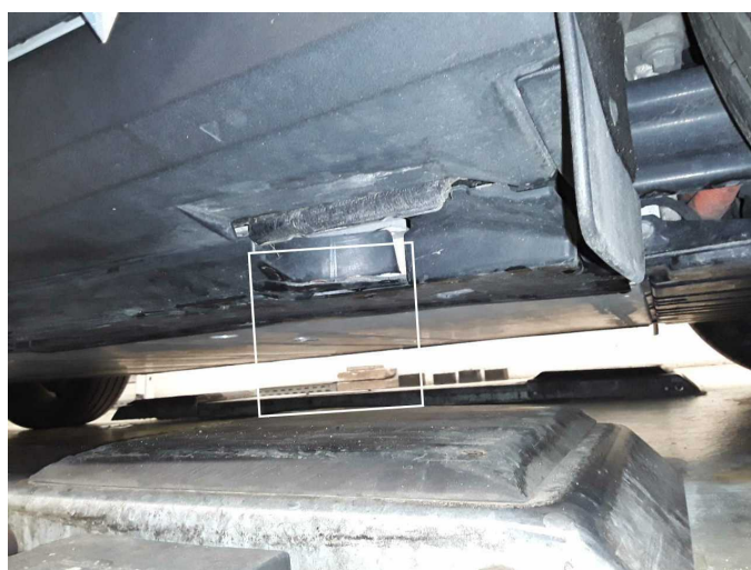
Damage 1: Body: Underbody panelling - Broken / torn - Replace
