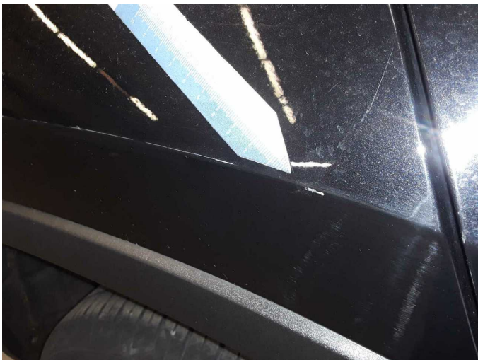
Damage 1: Side panel - rear right side: Side panel - Scratch(es) - Smart repair
