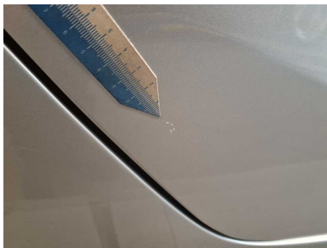
Damage 6: Door - rear right side: Door - Scratch(es) - Smart repair
