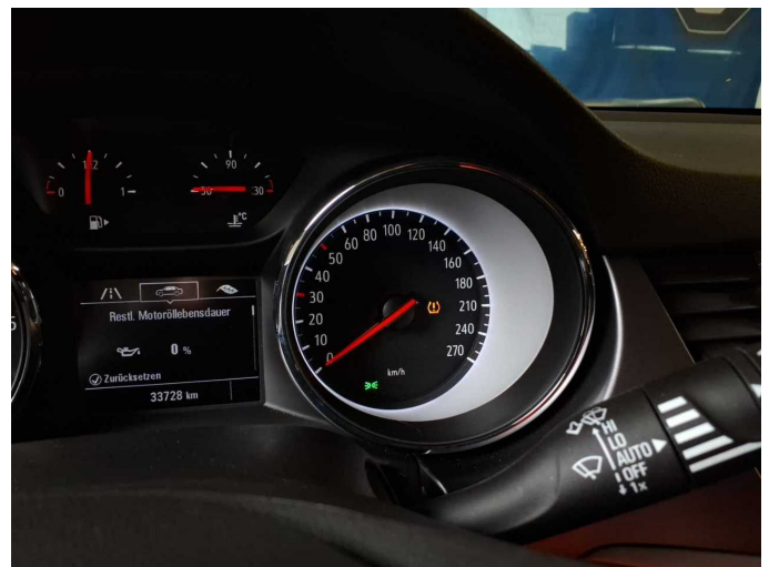
Damage 3: Wheel / tyres: Pressure sensor - on - Perform diagnosis
