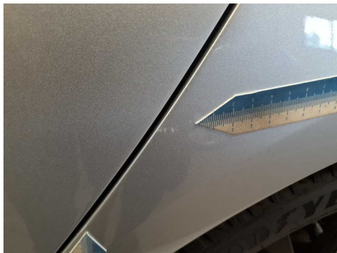
Damage 14: Side panel - rear left side: Side panel - Scratch(es) - Paint
