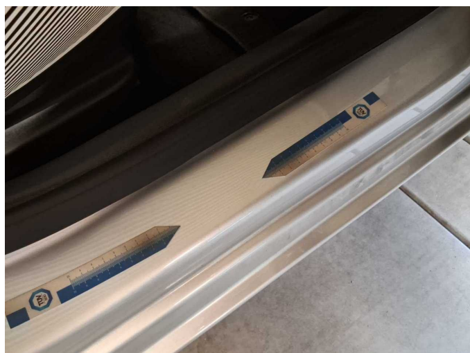
Damage 8: Sill - right side: Sill - dent(s) - Smooth repair work
