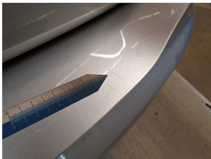
Damage 13: Rear bumper: Rear bumper - Scratch(es) - Paint
