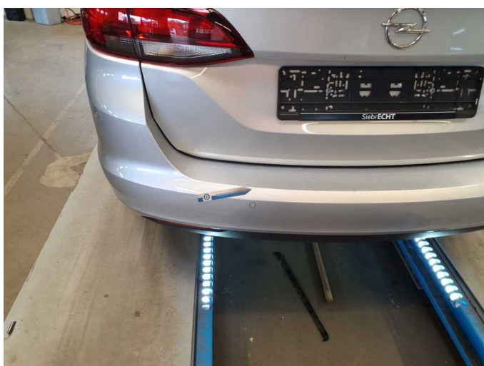
Damage 13: Rear bumper: Rear bumper - Scratch(es) - Paint
