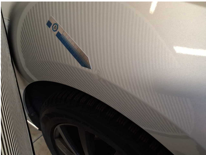
Damage 12: Mudguard - right side: Mudguard - right side - Dent / paintcoat damage - Repair and paint
