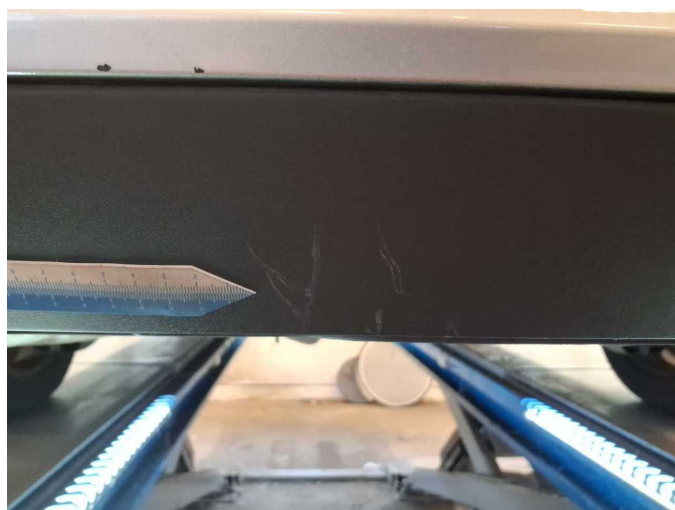
Damage 5: Rear bumper: Spoiler - Scratch(es) - Smart repair
