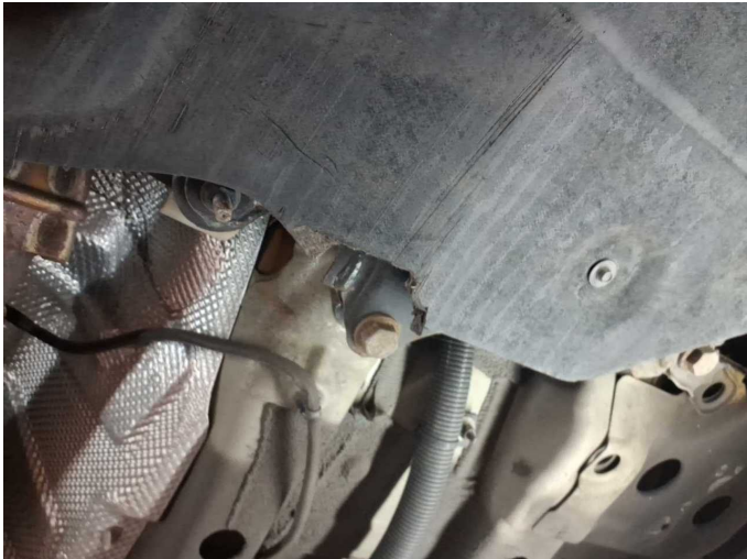
Damage 10: Engine: Engine cowling - lower - Broken / torn - Replace
