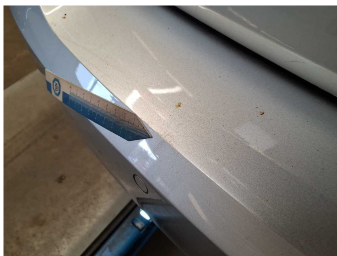
Damage 13: Rear bumper: Rear bumper - Scratch(es) - Paint
