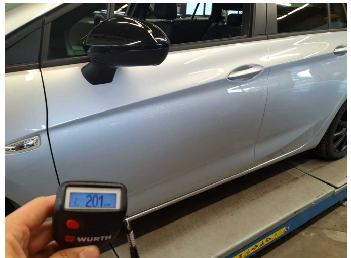
Repainting 4: Door - front left side
