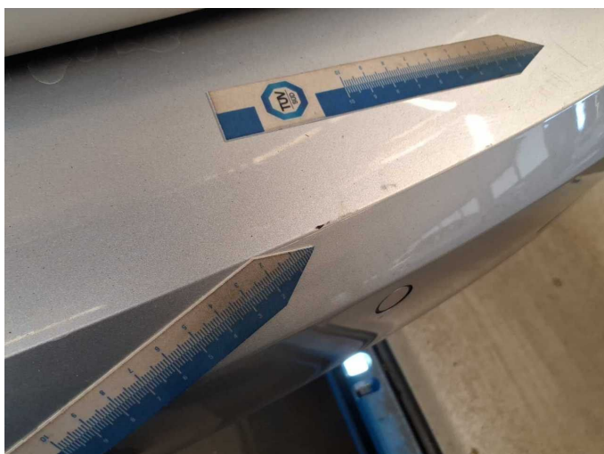
Damage 13: Rear bumper: Rear bumper - Scratch(es) - Paint
