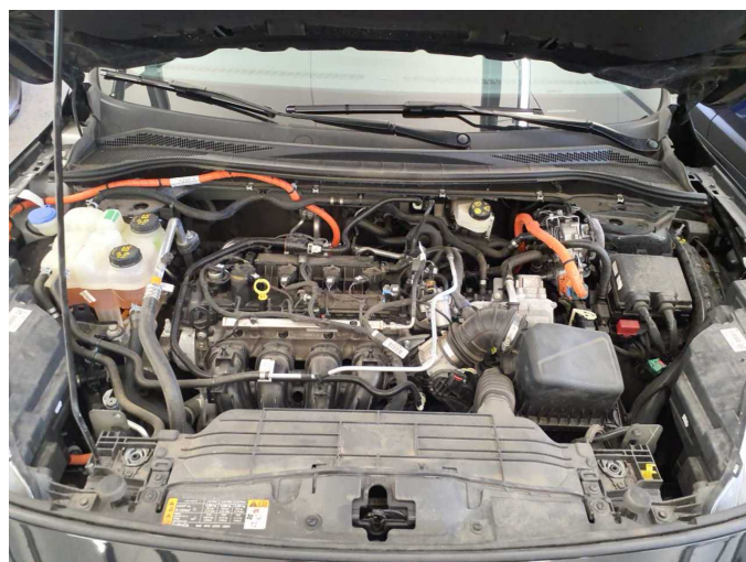
Missing part 1: Engine: Engine cover - Missing - Replace
